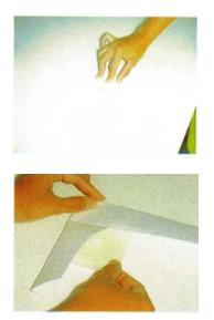
11. Cover the sample area on the sheet with a plastic plate for spreading and slowly push center of the plate to spread the sample.
